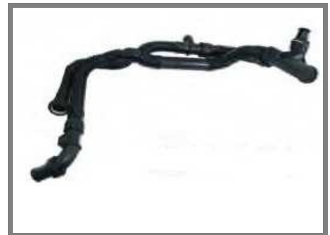
Water Distributer (Heater)
