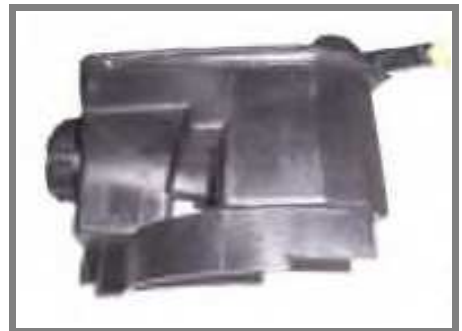
Steering Pump Box
